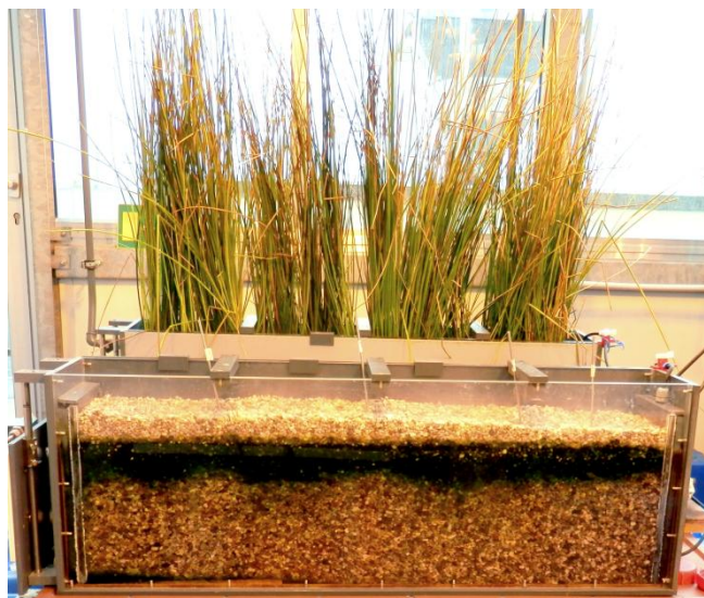
Figure 8: Photograph of the planted experimental laboratory-scale constructed wetland
