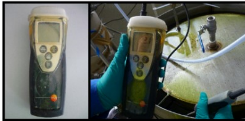
Figure 24. Measurement of gas temperature (by the author, 2014).
