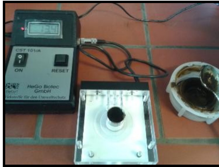
Figure 31. CST test for measuring sludge dewaterability (by the author, 2014).
