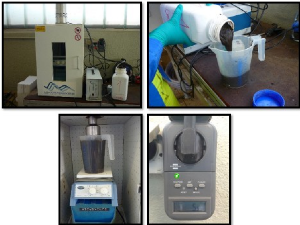
Figure 21. Application of the ultrasound treatment (by the author, 2014). The Ultrawaves ultrasound system used in the project was equipped with an oscillating unit consisting of a converter, booster and sonotrode (ULTRAWAVES GmbH, 2012b).
