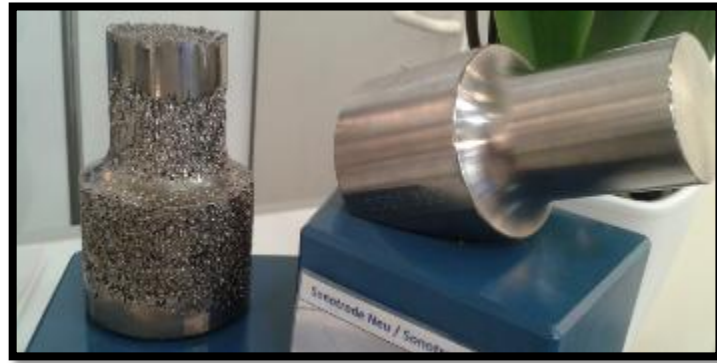
Figure 38. Comparison between a new sonotrode and one after three years of operation (by the author, 2014).
