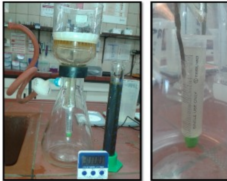
Figure 32. Set up for vacuum filtration test (by the author, 2014).
