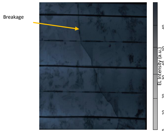
Fig. 1. EL image of a 15 cm x 15 cm polycrystalline Si solar cell.
