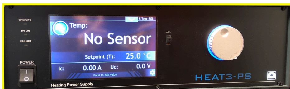
Figure 3.19 Temperature controller used for the thermal treatment of oxygen functionalized v-CNTs.
