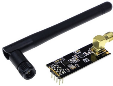
Figura 3.23: Transceptor de radio NRF24L01.
