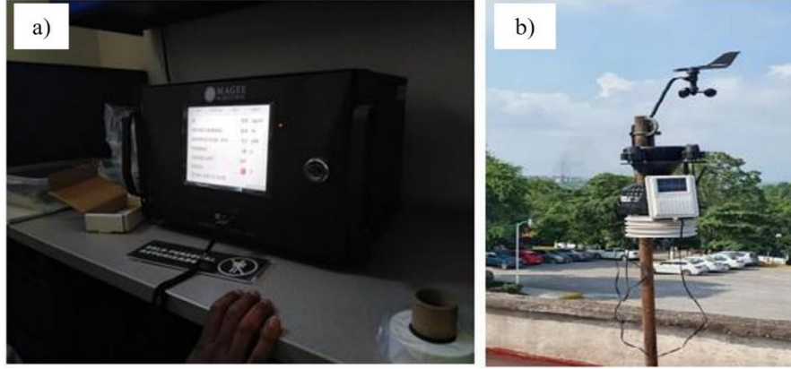
Fig. 4. Measuring equipment a) Aethalometer AE33 b) Mobile weather station Vantage Pro2.
